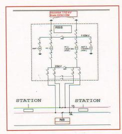
Simplified Scheme of Receiving Substation (RSS)
